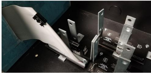
**Figure 26:** Ribbon cable routing example. After each cable is folded and folded as shown, their routed directly to the insulation and then run along the insulation until they reach the through hole shown on the left.
