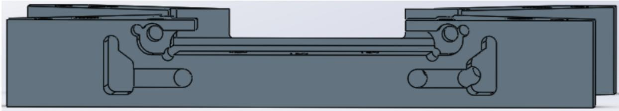
**Figure 17:** The back side of the shell with the connector slots.
